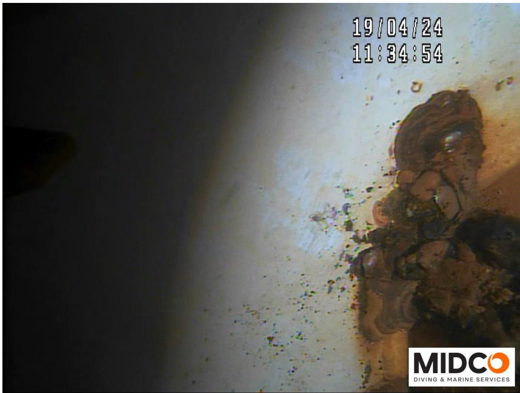
Interior Plumbing #1 – Coating Failure with Corrosion Noted
