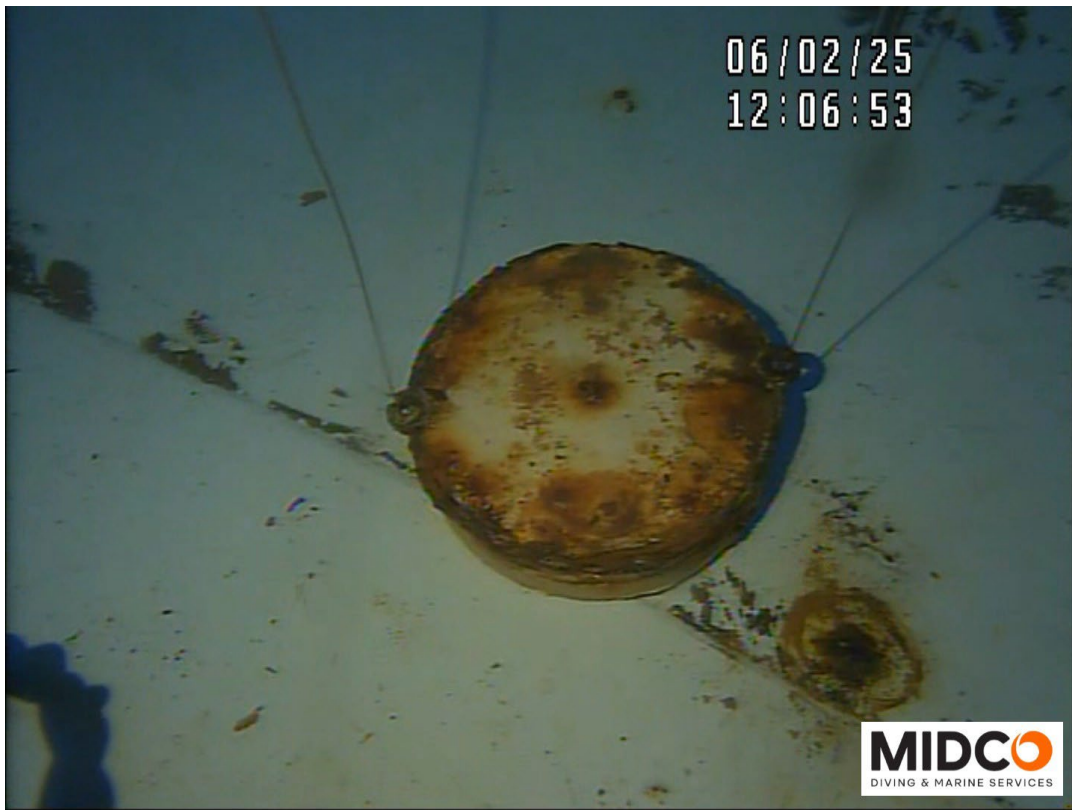
Manual Level Indicator Float – Non-Functioning
