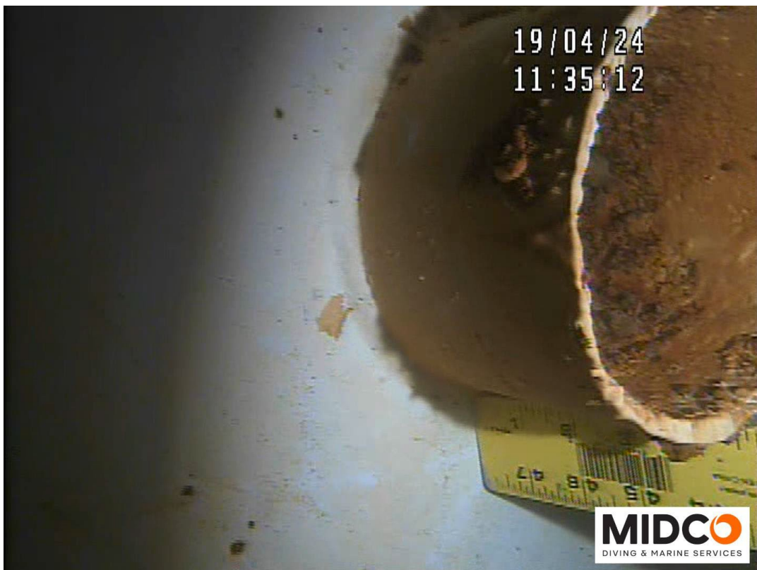
Interior Plumbing #2 – Coating Failure with Corrosion Noted
