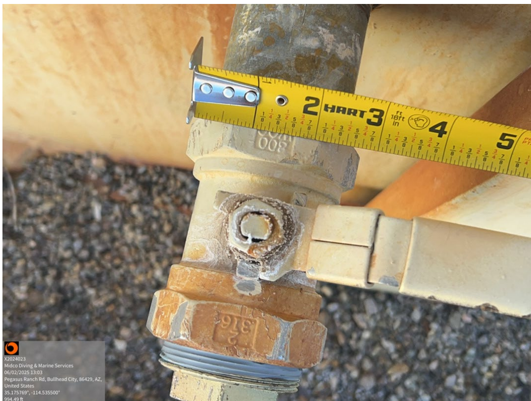
Water Tap – Coating Failure with Corrosion Noted
